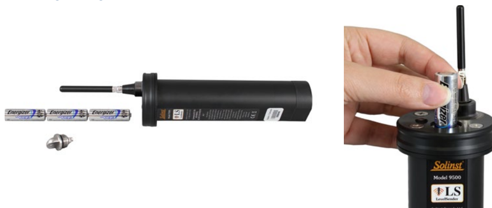
Figure 2-4 : Installation des piles
