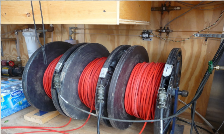
Transducer reels and flow meters
