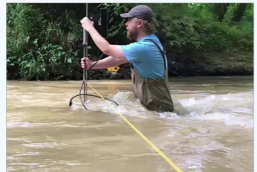
Conducting High Flow Measurements
