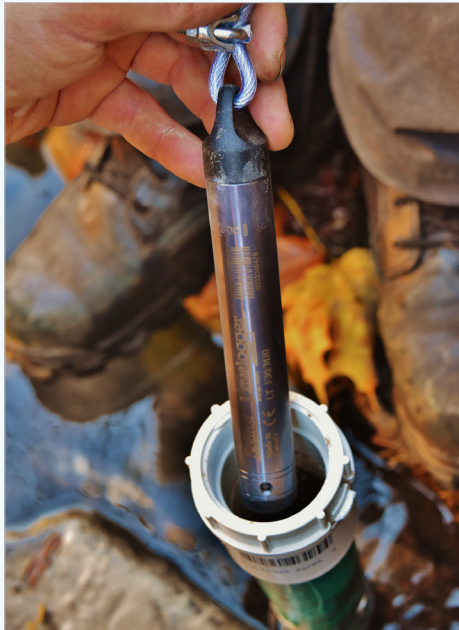
Levelogger Edge Installed in a Stilling Well
