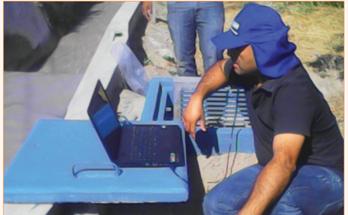
Water Level Data Downloaded in the Field Using a Laptop and Levelogger Software
