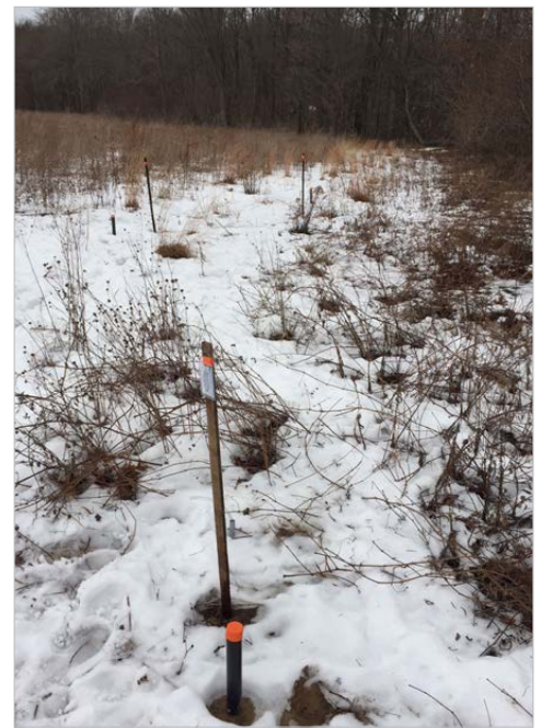
Groundwater Monitoring Wells Installed at Hibernaculum
