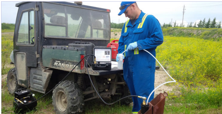
Bladder Pump Sampling Setup at the Newalta Stoney Creek Landfill
