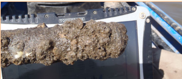
Levellogger fouled by Bay Barnacles and various other Invertebrates in the Hackensack River, NJ.
