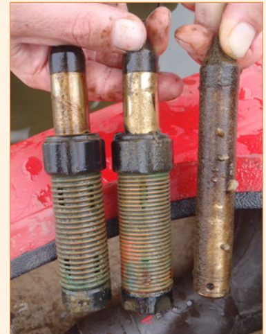
Little biofouling occurred on Levelloggers with Biofoul Screens. The control Levellogger had significant biofouling.
