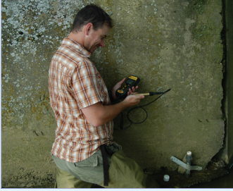
Photo at left: Duncan Gatenbee, an undergraduate research student, downloads data using a Levellogger Gold.
