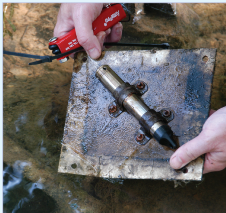
Levelogger installed flush with the streambed
