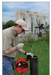
beam is refracted away from the detector which activates an audible tone and light.
