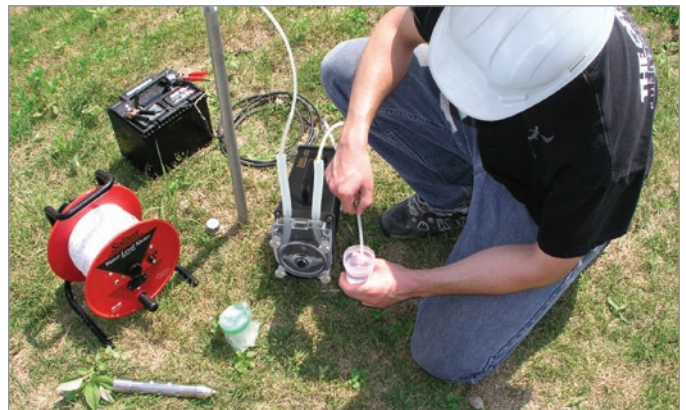
Sampling from a Solinst Model 615 Drive-Point Piezometer
