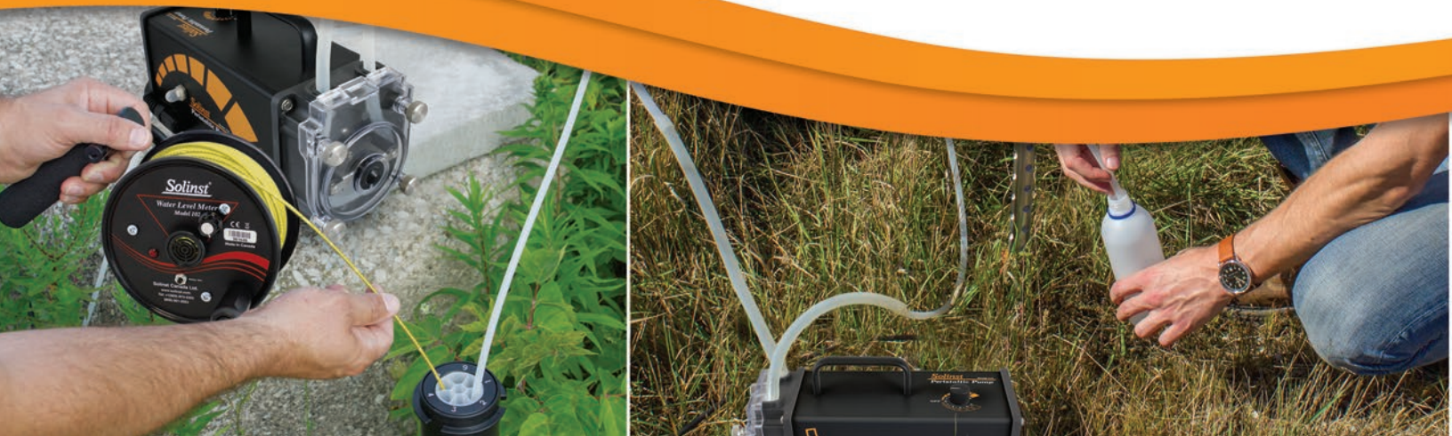
Sampling from a Solinst Model 615 Drive-Point Piezometer
