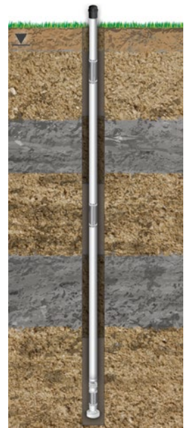
Typical 3 or 7-Channel CMT Installation using layers of bentonite and sand backfilled from surface.
