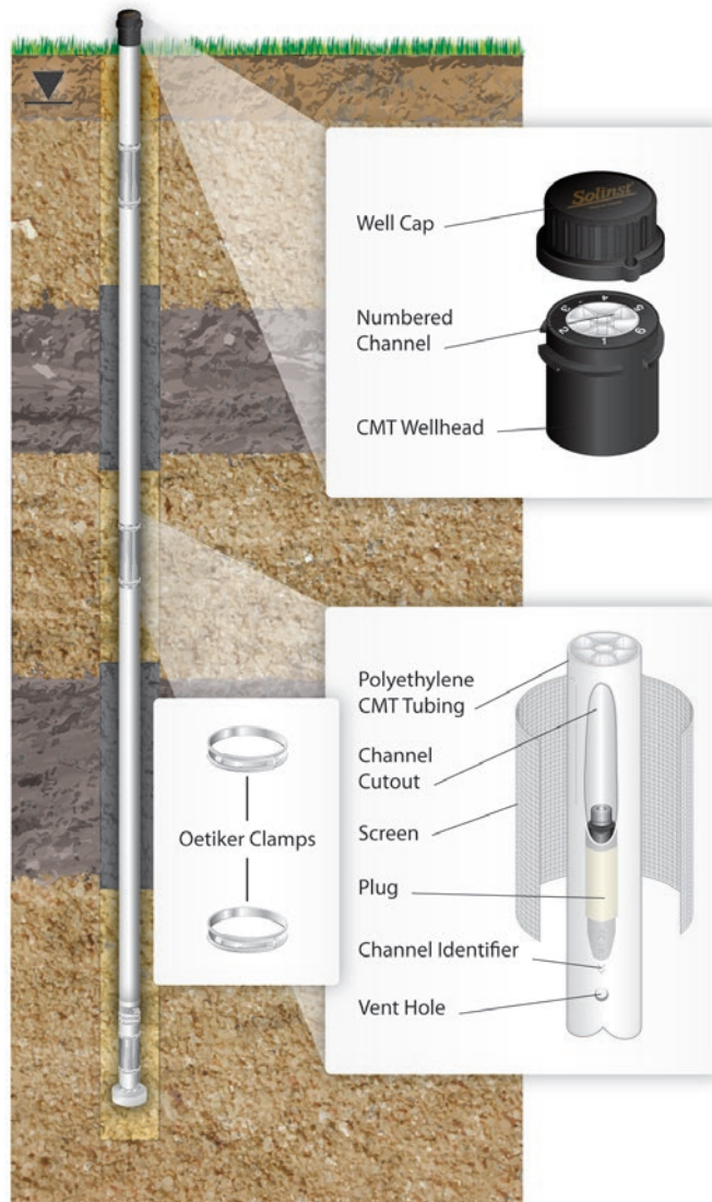
Typical 3 or 7-Channel CMT Installation using layers of bentonite and sand backfilled from surface.
