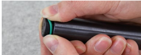
Figure 10-22 Replacing Levellogger O-rings
