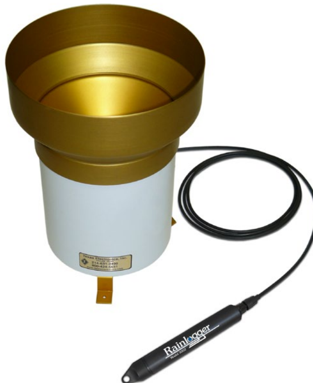
Figure 10-17 Rainlogger Edge Connected to Tipping-bucket
