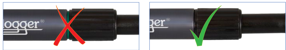
Figure 10-9 Proper Direct Read Cable Connection
