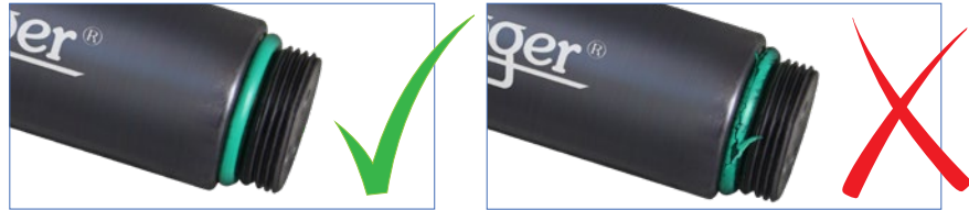
Figure 10-21 Levellogger O-ring Damage
