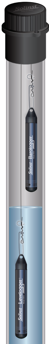
Figure 10-14 Levellogger and Barologger in Well
