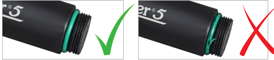
Figure 10-25 Levellogger O-ring Damage
