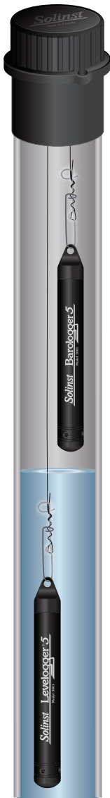
Figure 10-18 Levellogger and Barologger in Well
