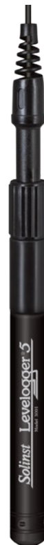
Figure 10-10 Levellogger 5 Connected to Older Style Direct Read Cable Using an L5-Edge DRC Adaptor
