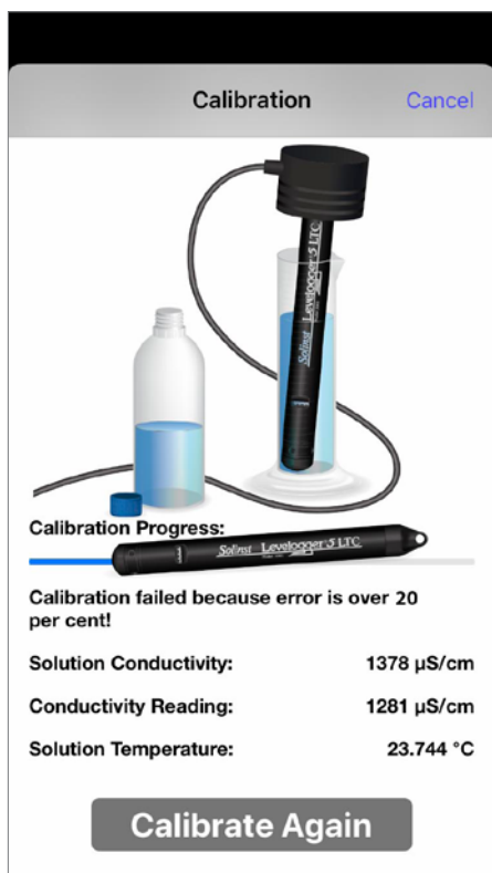
Figure 12-11 Conductivity Calibration Third Try - iOS
