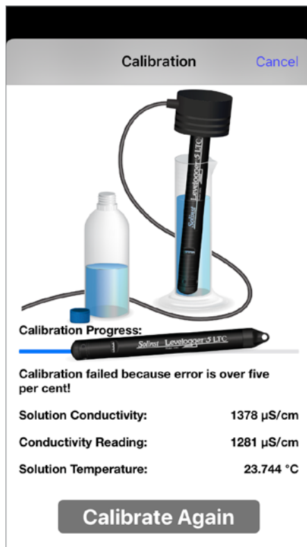
Figure 12-9 Conductivity Calibration Retry - iOS
