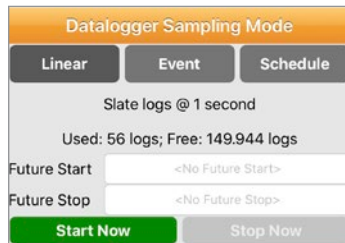
Figure 6-32 Starting and Stopping Dataloggers - iOS
