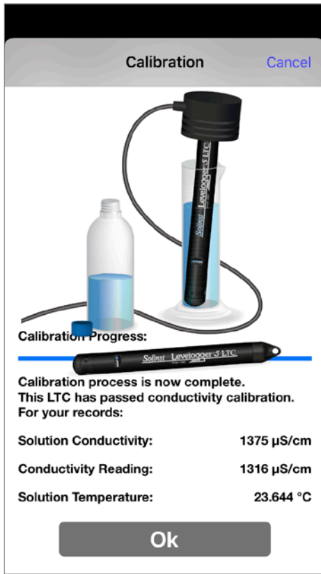
Figure 12-7 Conductivity Calibration Results - iOS
