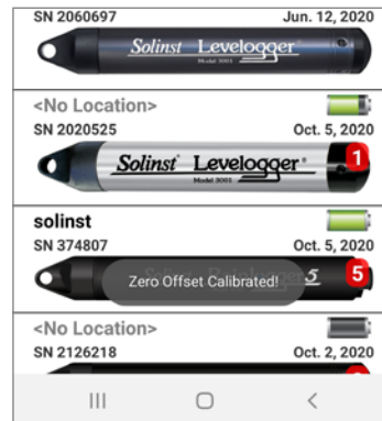
Figure 6-29 Zero Barometric – Android
