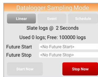
Figure 6-39 Stop a Logging Datalogger - Android
