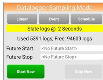
Figure 6-33 Starting and Stopping Dataloggers - Android
