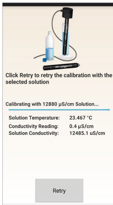
Figure 12-12 Conductivity Calibration Third Try - Android
