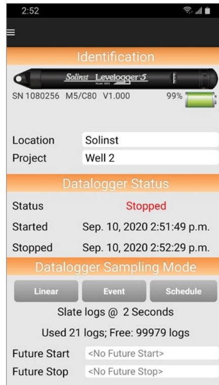
Figure 6-2 Edit Datalogger Settings - Android
