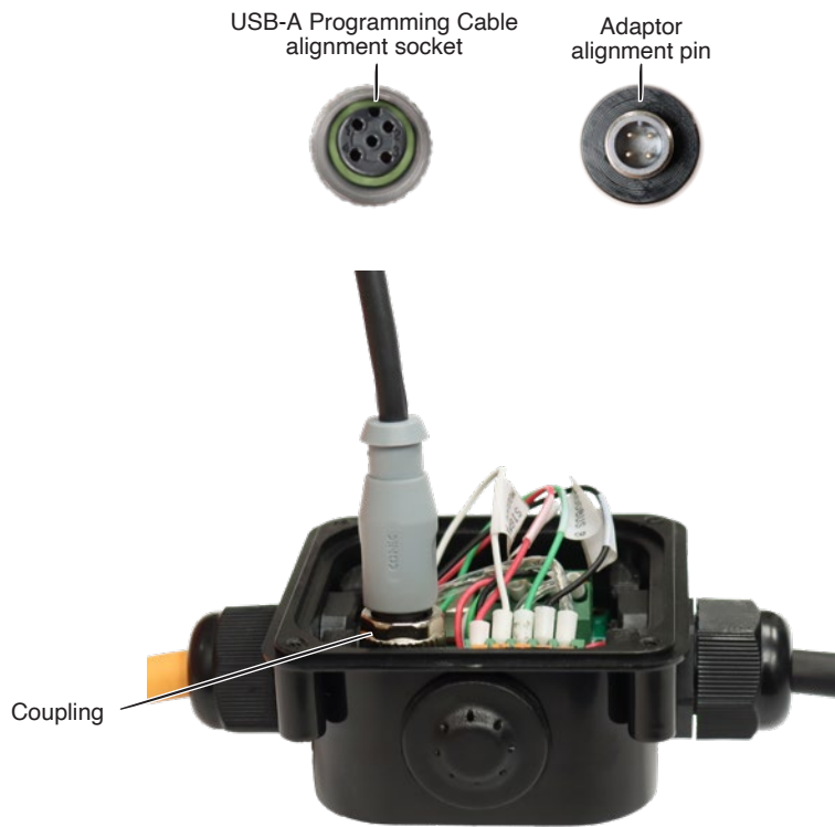
Figure 2-1 Connecting the USB-A Programming Cable
