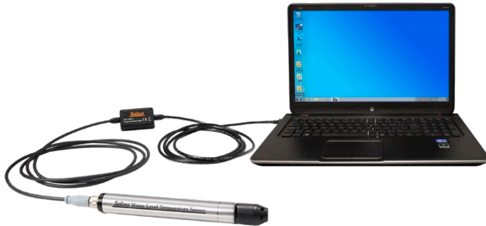
Figure 2-2 WLTS Utility Communication
