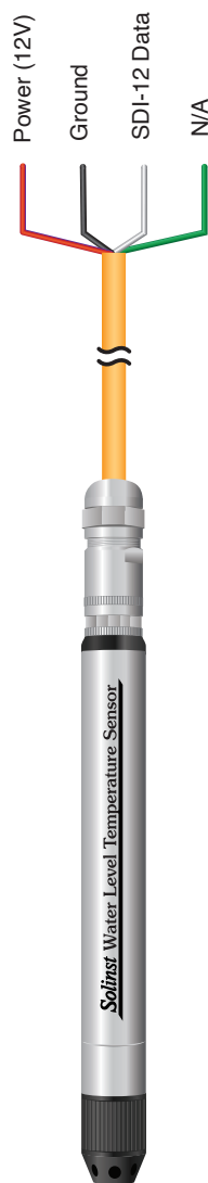
Figure 3-1 WLTS SDI-12 Wiring Overview
