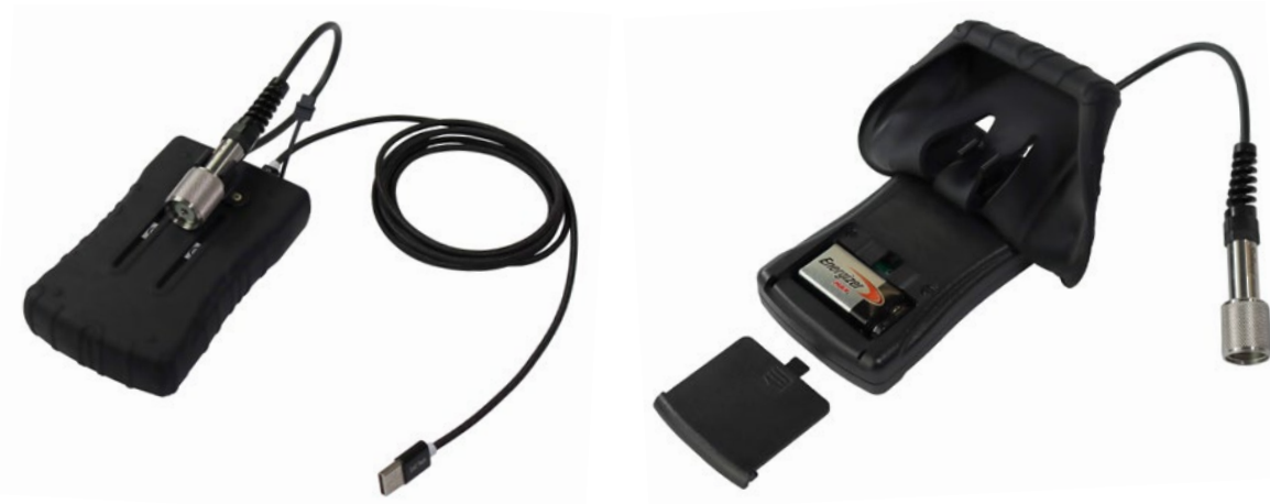
Figure 8-1 SRU Battery Installation
