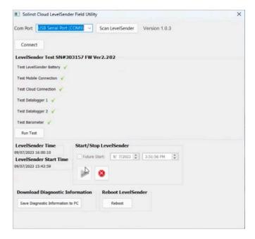
**Note:** The Firmware Upgrade Utility is downloaded along with the Solinst Cloud LevelSender Field Utility. See the LevelSender 5 User Guide for firmware update instructions.
