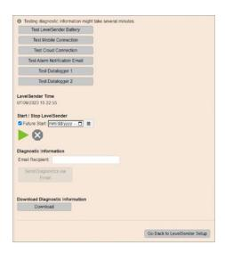
You can test the LevelSender battery, mobile connection, Cloud connection, alarm notification email, and dataloggers.
