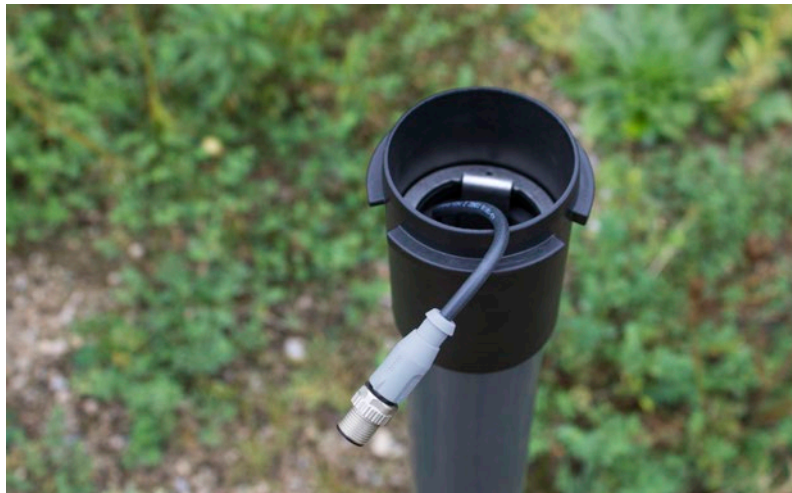
Figure 6-6 Lower the Assembly into the Well
