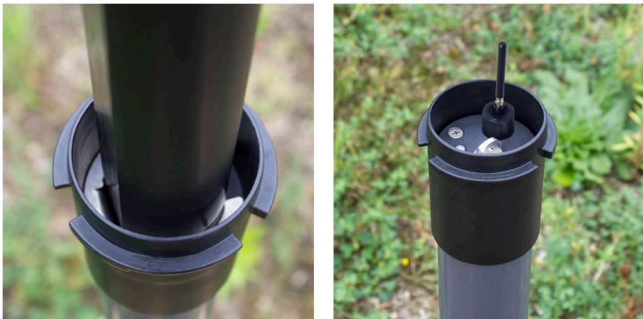
Figure 6-8 Lower the LevelSender into Position
