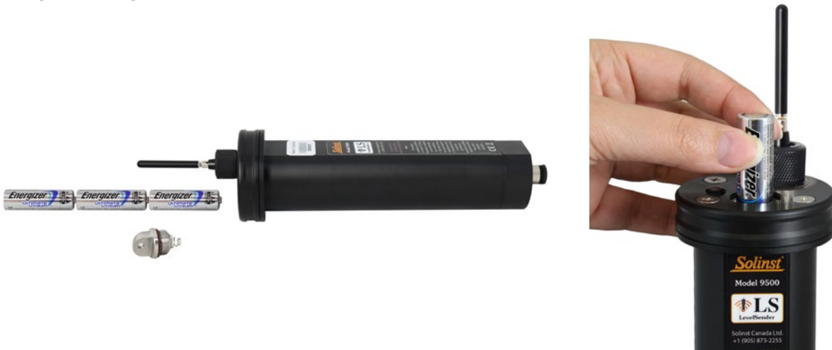
Figure 2-4 Installing the Batteries
