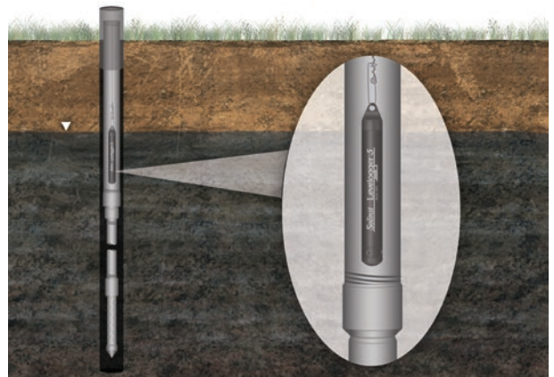
Levelogger Installation Just Below Lowest Expected Water Level
