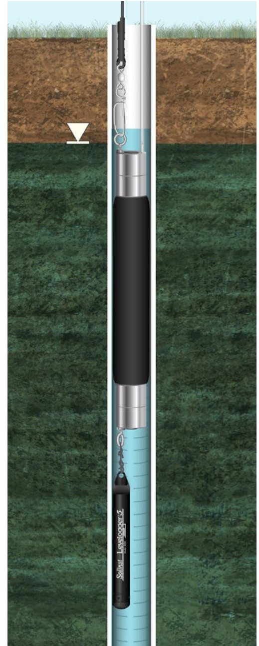
Solinst Model 800 1.8" OD Single Point Packer Falling Head K Test Setup in 2" OD Well
