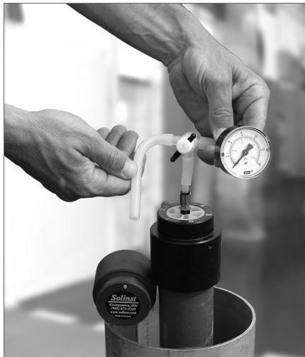
7-Channel CMT fitted with a three-way valve used for vapor sampling.
