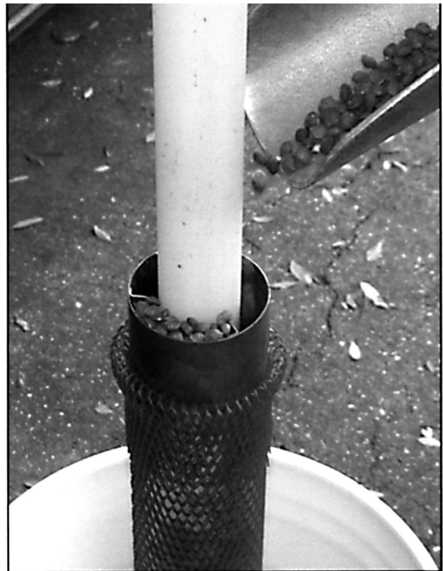
Figure 6. Stainless-steel form used to construct bentonite packers.
