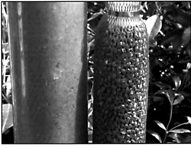
Figure 7. Bentonite packer (right) prior to insertion in a borehole. To left, bentonite packer after it has hydrated and swelled.
